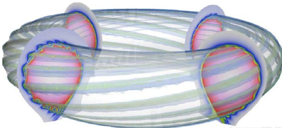
Non-linear MHD modelling of plasma edge relaxations due to Edge Localized Modes (ELMs) in a tokamak using JOEUK code (courtesy to G. Huijsmans)
