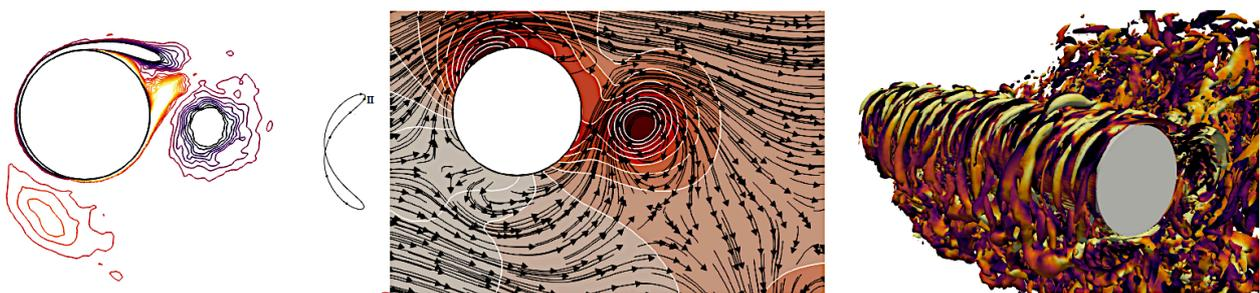
**Figure 1.** Span-phase-average iso-contours of span-wise vorticity at sub-critical regime and  $U^* = 5.5$  (left column) and pressure (center column). Instantaneous flow visualisation by means of  $Q = 3.0$  iso-surfaces coloured by stream wise vorticity (right column).
