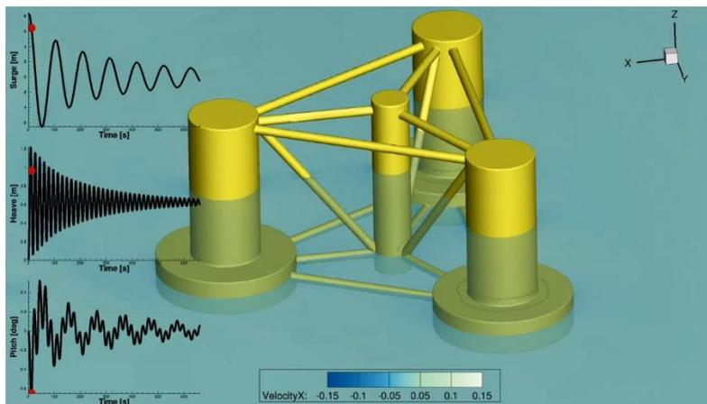
Fig.1 – Unsteady non-linear RANS calculation of a Floating-Offshore Wind Turbine Platform. Calculation took around 3 weeks in 200 cores of a modern HPC cluster. Click for [animation](#).
